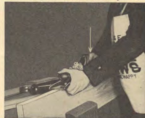
Fig. 30—Making a glue joint. One piece in vise. Note how plane is carried straight, with fingers under it to guide, thumb on knob, and pressure on rear of plane at arrow.
