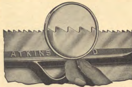
Fig. 51—Shows Rip Saw teeth ready to file. After jointing, shaping and setting Rip Saws, the pitch in rip teeth should be as shown in this illustration.
