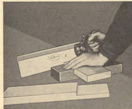
Fig. 13—Cutting shoulders of half lap joint with ATKINS Silver Steel Back Saw No. 2, in bench hook.
