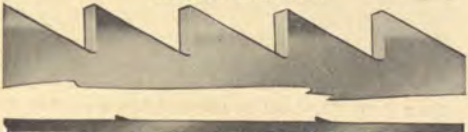
Fig. 5—Side and top views of RIP Teeth of a hand saw.
