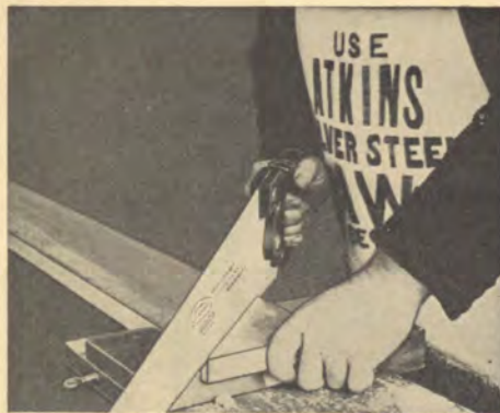
Fig. 18—Cutting a mitre joint with ATKINS Silver Steel Panel Saw No. 58.
