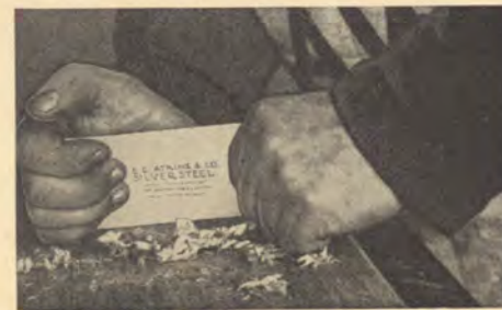
Fig. 42—Using an ATKINS Silver Steel Scraper Blade on hard wood, in building wall tool cabinet.
