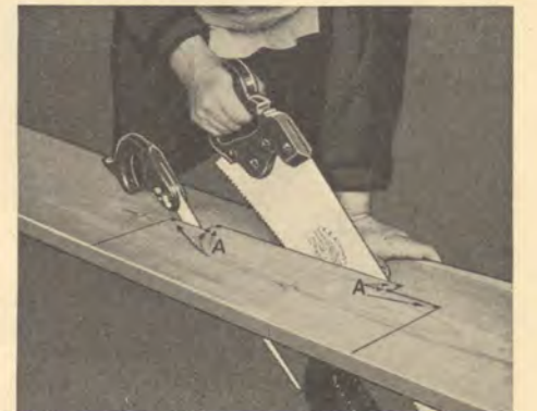
Fig. 40—Cutting drawer opening and hand hole in bench apron with ATKINS Silver Steel Rip Saw; showing ¾" holes bored at A, and the use of ATKINS Compass Saw in starting the cut.
