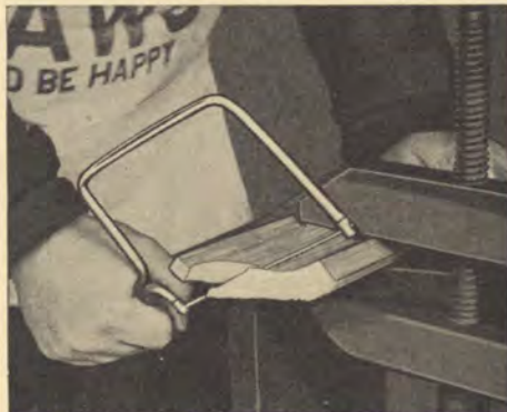
Fig. 35—Using the ATKINS Silver Steel Coping Saw No. 100 to cut moulding for a coped joint.
