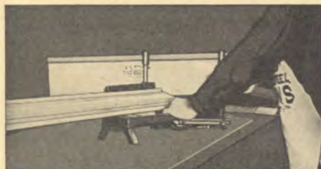
Fig. 19—Using ATKINS Silver Steel Mitre Saw No. 1 to cut moulding in a mitre box.
