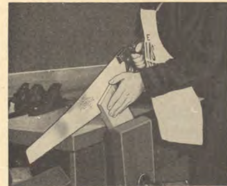
Fig. 14—Making depth cut of half lap joint with ATKINS Silver Steel Hand Rip Saw No. 53.
