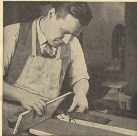
Fig. 1—The quick, easy way to cut grooves is with an ATKINS Silver Steel Dado Head on your bench machine.
