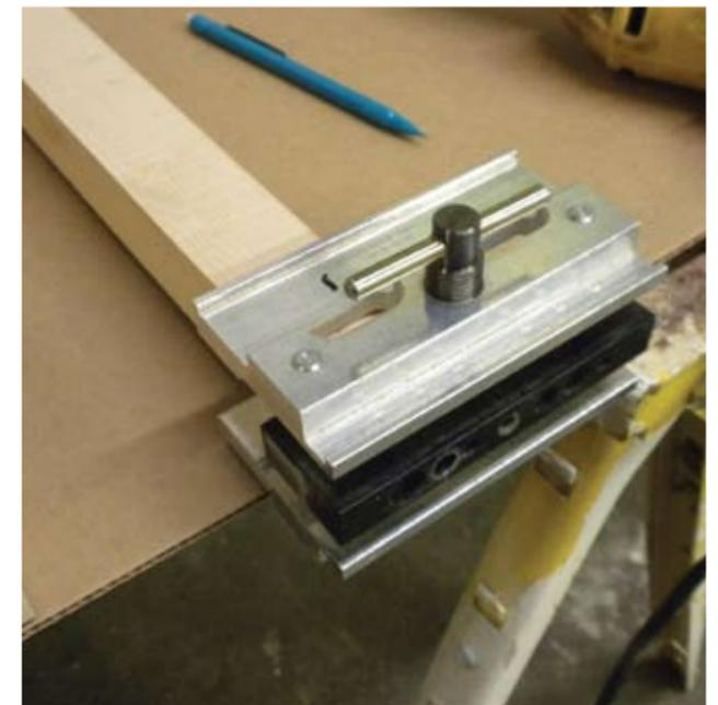
**4** This dowel jig is worth its weight in gold, and at \$40 it is one of my favorite bang-for-your-buck tools. It automatically centers the hole across the width of the parts and accepts thick stock such as these legs and stretchers.
