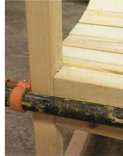
10 I used a 2x4 stretcher at the front of the bench to join the sides — this may be overkill, but it provides a lot of rigidity. I also added an identical one to the back of the bench.
