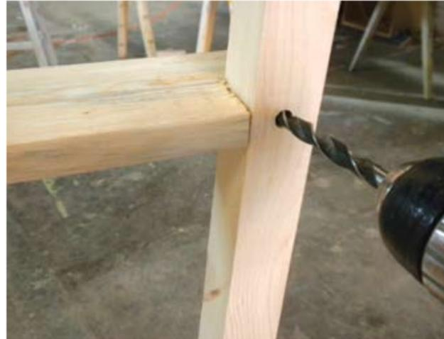
16 The back of the arm is easy to attach to the rear leg with a long, counter-bored screw.
