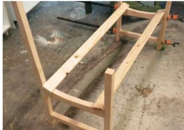
7 (ABOVE LEFT) With the first side clamped up, the second goes together the same way — and it is usually a little bit quicker, as well, since you've just practiced it once. I like to lay the parts on top of the first side to double-check that the sides are identical and that no errors crept in the second time around.
