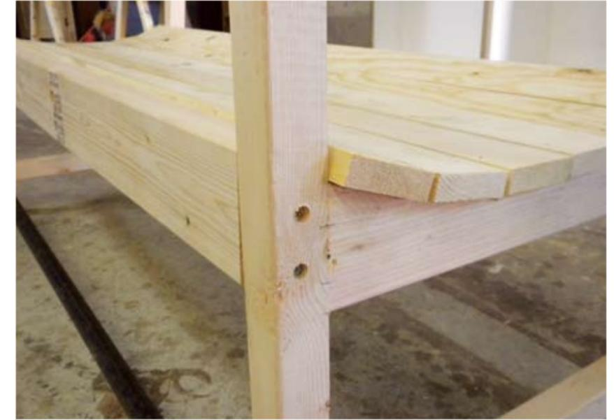
11 The stretchers are positioned so that their top edge is essentially flush with the seat slat closest to them. I secured the stretchers with long screws.
