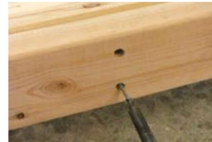
17 (ABOVE LEFT) To provide a safe and sturdy seat, I attached a brace on the underside of the slats. The profile matches the curve on the stretchers that hold the sides together.
