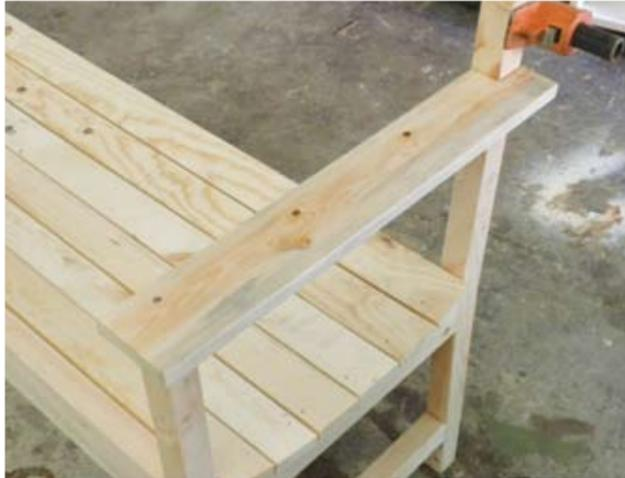
15 The arm can be attached to the front leg by simply screwing down through the top of the arm.
