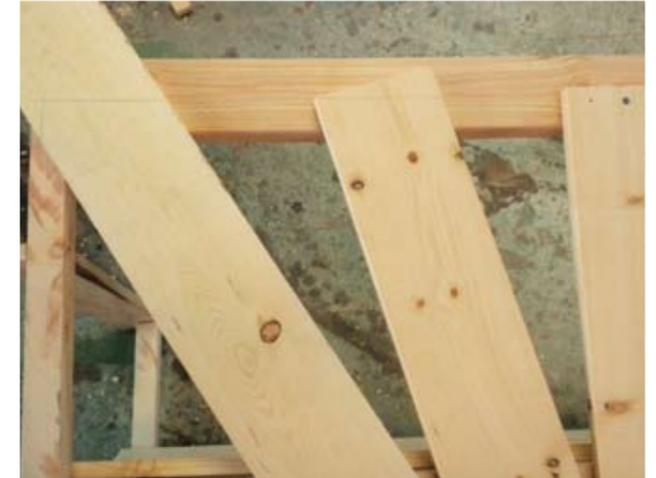
21 I also drew a line across the top. The top corner of the slat on the end needed to be trimmed to a point.
