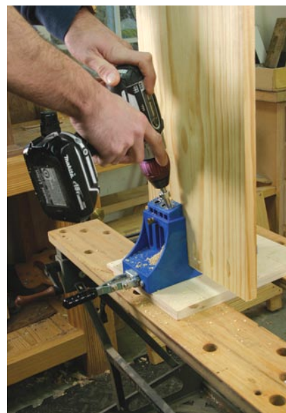
Screw this. The entire project is assembled with pocket screws. Here I'm boring five pocket holes on one end of the back piece.
