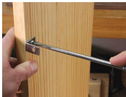
Stops sagging. Don't forget the little L-brackets under the top. These prevent the top piece from sagging.
