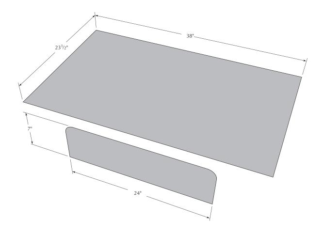
Sew seat fabric to sides, wrap around cushion assembly and staple to bottom edge of frame
