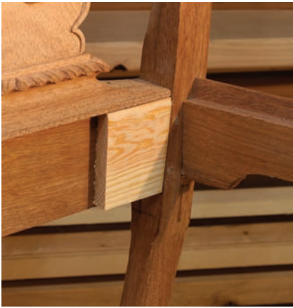
Add fillers as needed. Filler blocks were used to flush the rear seat rail to their adjacent legs. Some fillers stretched across the entire rear rail. Some chairs didn't need fillers.
