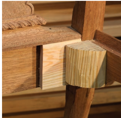
Simple blocks. The corner blocks were made up of two laminations of 4/4 pine. I didn't see any thought as to grain orientation beyond that they ran parallel to legs. The pieces didn't seem to be quartered or riven.
