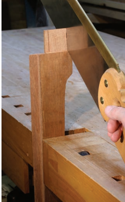
Wedge prep. Repairs and X-rays done at the Philadelphia Museum of Art indicate 18th-century Philadelphia chairmakers sawed their tenons in preparation for wedges.
