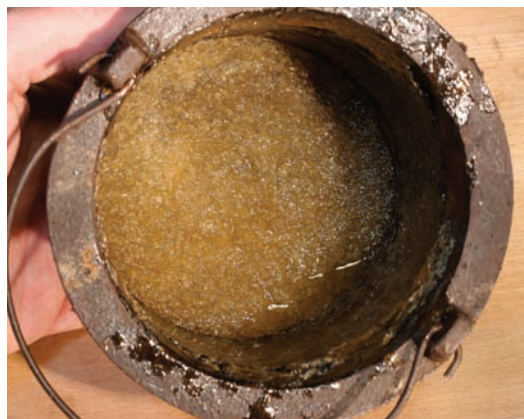
Hot and sticky. I cover the bottom of my glue pot with dry glue. Then I pour in cold water to cover it. The dry glue quickly absorbs the water and becomes a gelatinous mush. Ten minutes later, I look in the pot, and maybe add a bit more water. In an hour it looks like this. The glue has absorbed all the water it cares to. A little excess water is present. Were there a cup of excess water, I would try to pour it off. The glue is gloppy, not runny at this point. Or you could forget about it and cook the water off.
