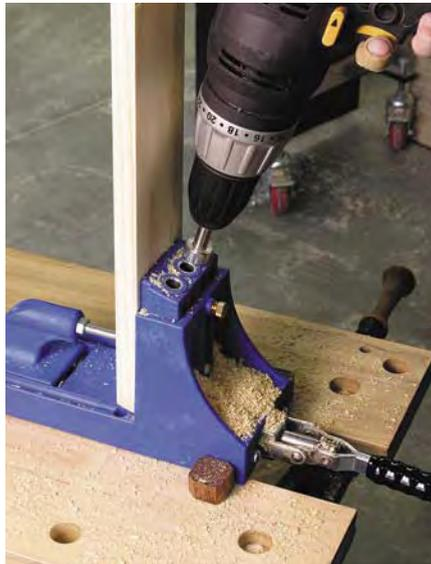
After securing the board firmly in the jig, squeeze your drill's trigger and allow it to get up to speed before drilling into the wood.
