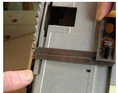
Properly set. A plunge-cut saw is set up with the blade slightly canted at the front. Here you can see the paper-thin gap needed to make a saw work its best.
