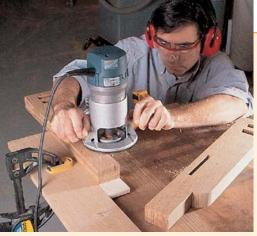
When pattern-routing the curve on the legs, make sure you have the work firmly clamped in place. I have the pattern and leg wedged between two pieces of oak (the pattern is on the underside of the leg). Then the leg itself is clamped to the table. You also could perform this operation on a router table with a starting pin for pattern-routing.
