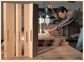
Make the mortises in the legs before you shape the curve near the bottom or make cutouts on the top.
