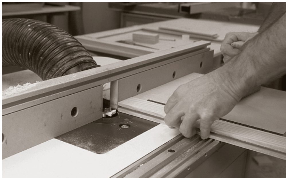
When cutting the tenons, hold the part down firmly against the edge of the back-up block and tight to the router table fence. Guide the part using
