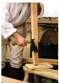
I like to brag about how roughly and quickly I work because I think it marks a significant departure from my perception of "Norm-al" woodworkers. The truth is, this is only the first step. I start rough, then refine where needed. In this picture, I'm producing the leg taper with a hatchet.
