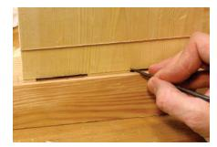
I mark the tenons directly from the mortises. It's important to have nice crisp ends on your mortises. When the ends are rounded over even a little bit, it's tough to know how wide to make each tenon.
