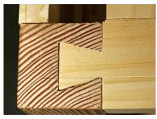
The upper rail holds the tops of the two front legs together. I think the trick to getting any dovetail tight is sawing accurately. Beyond that, what you want is for that wedge shape to pull against the shoulders. If the top is too tight, the wedge shape can't do its job. So I shaved away a bit of the top of the tail to get a tight fit. This joint won't be visible in the finished piece.
