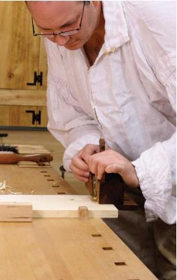
It's tough to saw tenons on a wide board. I'm using a fillister plane instead. The disadvantage of this method is that the shoulder of the tenon is defined by the end of the board (where the plane's fence rubs). That means the length of the board must be just so. So this isn't a better way to cut tenons, but it's a reasonable alternative for wide carcase sides. See my blog for a demo.
