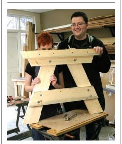
**Ends are the beginning.** Make the two end assemblies first. Then attach the top and diagonal braces.
