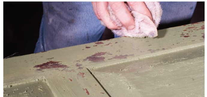
Use a wet cloth to wipe away paint in areas as the paint begins to dry. Try to best simulate wear areas based on antique originals.
