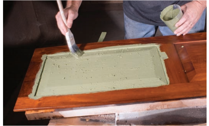
An old look for paint begins with a small amount of sawdust in the paint and the mixture applied to the project. Work in small areas to keep the process from getting away from you as it dries.
