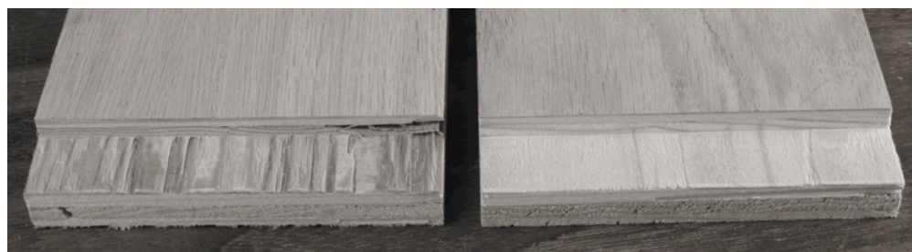
The differences in core materials may not be apparent until you make a joint. The fir core at left chipped severely while the hardwood core at right had a smooth surface.
