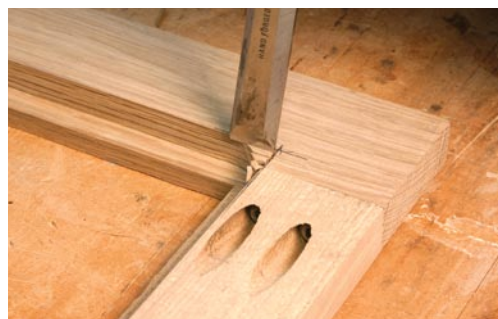
Squaring the corners left rounded from the router bit is a job for the chisel. It works best to begin with a cut across the end grain and to then take small cuts with the grain, removing the waste.
