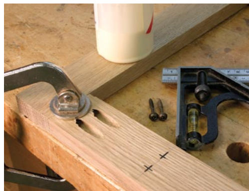
Positioning the pocket-screw holes in the door rails is important. Too close to either edge can cause problems. Don't forget to add glue at the joint.
