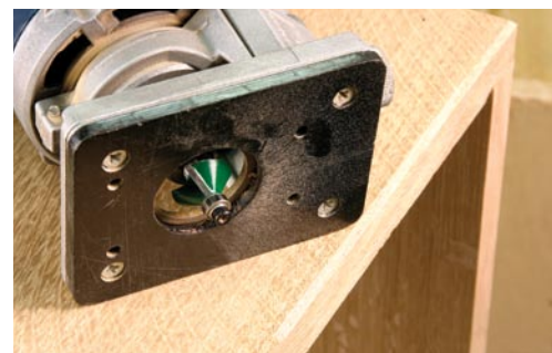
Adding a small bevel to the edges of the piece will help hide the joints between the separate units. This edge work also allows the doors to flip up and slide back into the case without binding.
