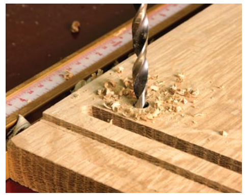
There are pin locations at both the top and bottom that act as guides for the doors. Use the drill press for this step – unless you've a steady hand and good eye.
