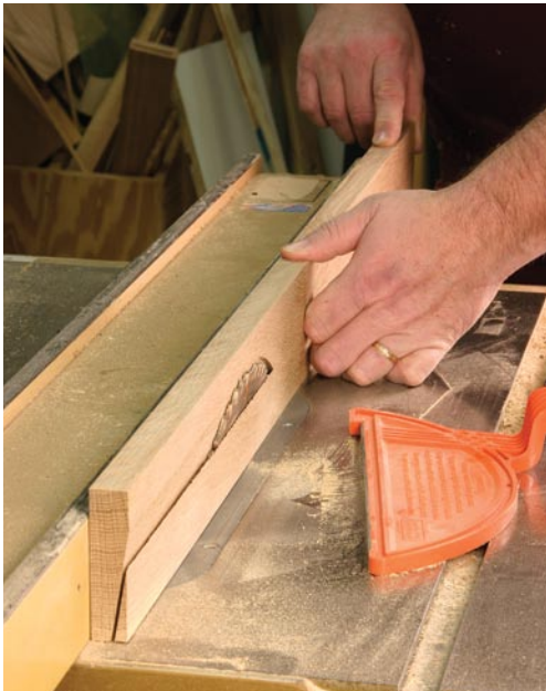
The cutting of the crown moulding can leave saw kerf indications and burn marks. A quick run over the jointer knives works best to clean the face.
