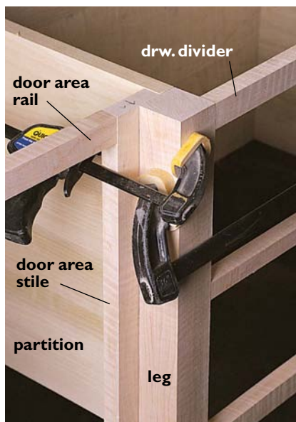
The most complicated joinery location on the piece. Shown here is the intersection of the left, middle leg, with the partition, top drawer divider, and left door section stile and top rail. Once you get a good look, you can see it's simple.
