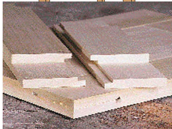
The door section bottom is a half-lapped frame and panel. Seen from the ends, the two frame pieces show the center groove for the panel, and the half-lap cut. Seen below the pieces is the assembled frame (left).
