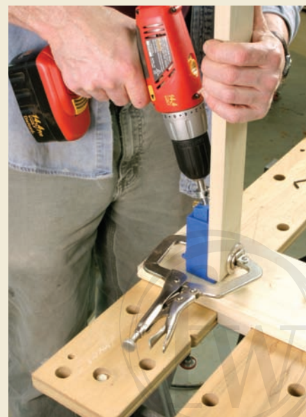
Use the high speed setting on your drill to make the pocket hole.
