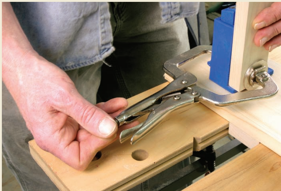
Adjust the clamp to hold the wood firmly in the jig without taking too much effort to set the clamp.
