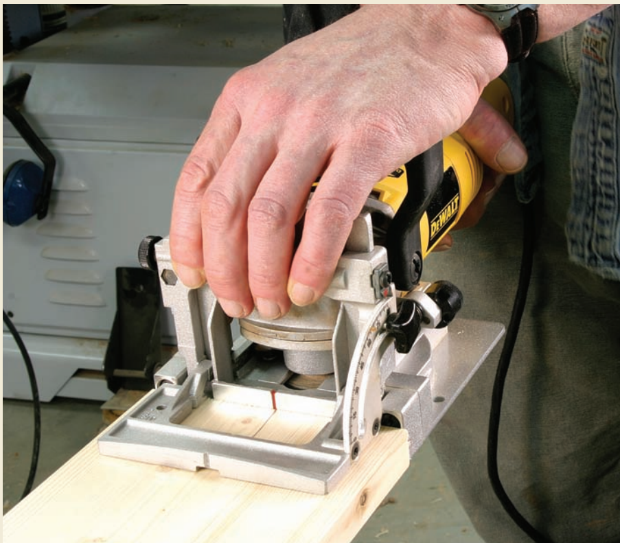
An alternate way to plunge: Squeeze the fence and tool handle together to make the cut.
