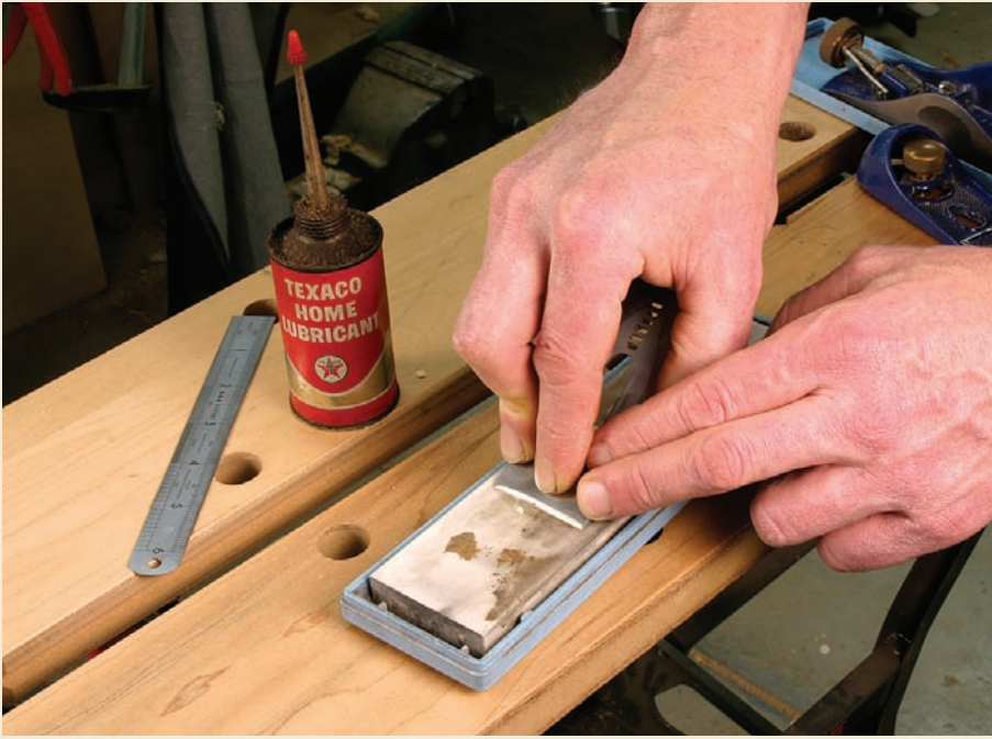
Learning to hone the bevel takes a little practice. Take it slow and check your work frequently. A honing guide is a good $12 investment if you can find one at your home center.
