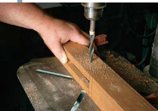
Try to do as much work on the posts – mortising, drilling, etc. – before you cut the octagonal tapers.
