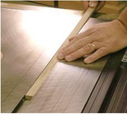
**Follow the guide.** The guide is a key component of the sled. The accuracy of the fit to the table slot is paramount in attaining a square cut. A sloppy fit equals a sloppy cut.
