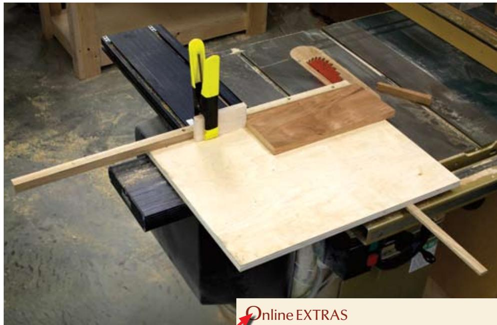
**Repeatable, perfect 90° cuts.** Cutting panels with a standard issue miter gauge is "iffy" at best. While the degree of difficulty to build and use this panel-cutting sled is near zero, the results are a 10.
