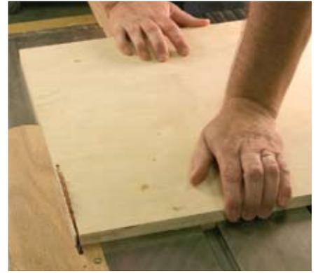
**Getting the accurate edge.** Sawing the edge of the jig after the guide is attached to the panel ensures the edge is parallel to the blade as well as the guide.
