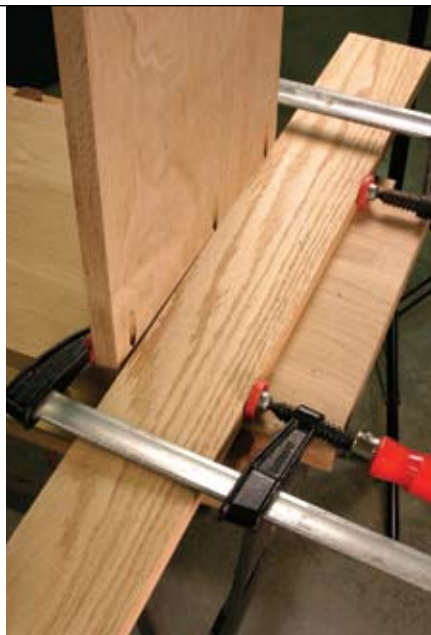
You can pull a cup out of a board by clamping the piece to a straightedge and pulling it tight with clamps before screwing it down.
