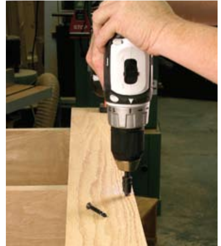
Make sure your drill is at a 90^\circ angle to the most narrow stock through which you're drilling – in this case, the \frac{3}{4} " edge of the side beneath the support.
