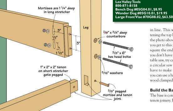
end assemblies that are joined by two rails. The end assemblies are built using big 1"thick, 2"-long tenons. The front rails are attached to the ends using 1" x 1" mortiseand-tenon joints and the 6"-long bolts.
