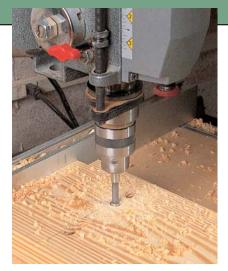
The mortises in the front rails are also made on the drill press. Make them  $1\frac{1}{4}$  deep to make sure you can get a washer in there. If you can't, try clipping an edge off of the washer.
