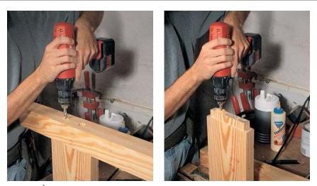
Drilling the <sup>3</sup>/8" holes for the bolts is easier if you do it in this order. First drill the holes in the legs using your drill press. Now assemble the leg and front rail. Drill into the rail using the hole in the leg as a guide (left). Remove the leg from the rail and continue drilling the hole in the rail. The hole you drilled before will once more act as a guide. You still need to be careful and guide your drill straight and true (right).
