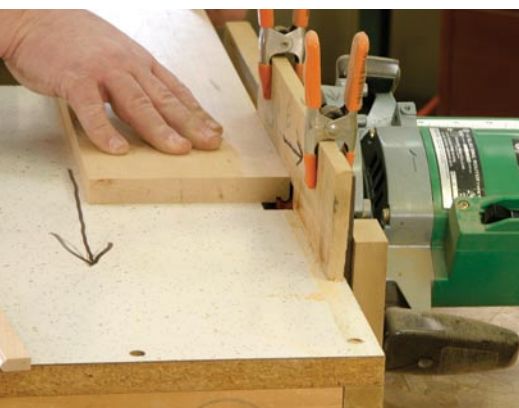
A smooth face. Flatten the edge of the stock with a handplane or jointer before milling the bead. This guarantees a "show" face on the bead. Make certain to install the smooth face outward.
