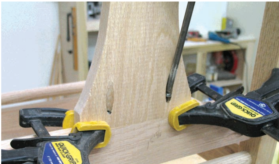
With the splat held flush to the back face of the legs, the pocket screws are driven home, finishing the assembly of your stylin' chair.
