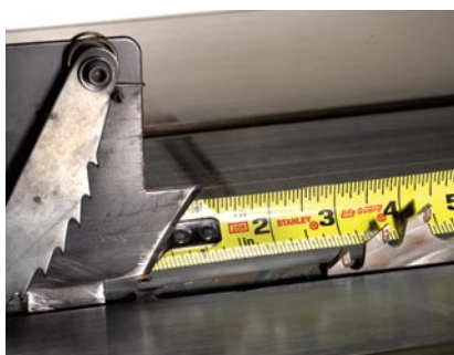
Dangerous gap. Standard splitters do not follow the blade as it raises or lowers. Therefore, the gap between the two can be wide. This opening is an area where pinching and kickback can develop.
