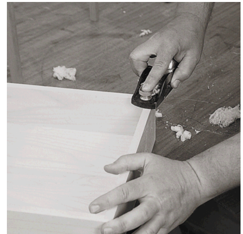
The first step in fitting the drawer is to trim the height. A simple block plane can be used to take off a little bit at a time until the fit is perfect.
