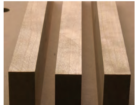
Not glue ready. The edges produced with plunge-cut saws are clean, but in the rake of the light, small saw marks can be seen.
