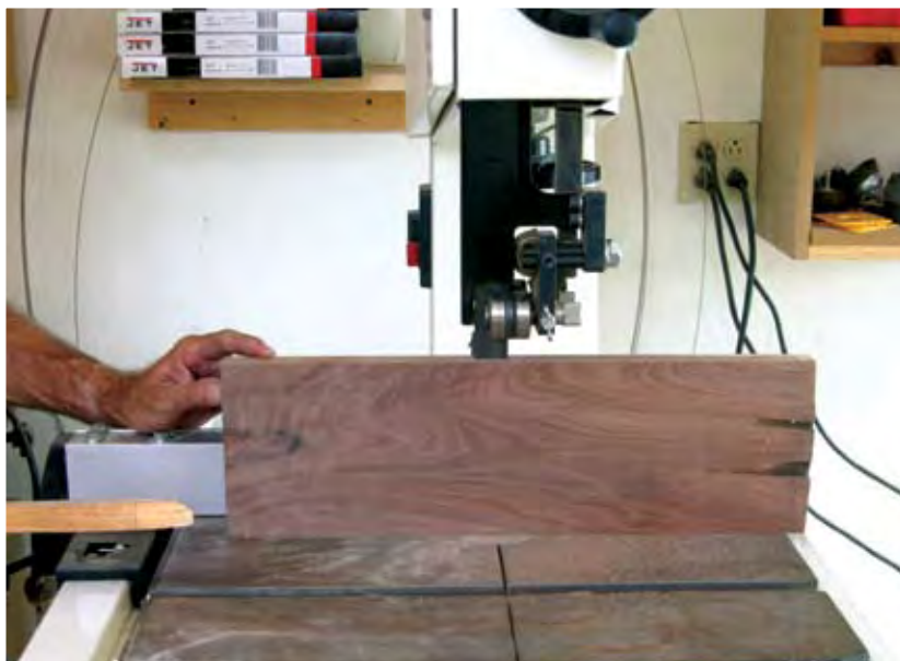
Band saws can also be used for resawing thick stock into thinner stock. The Jet model shown features a bolt-on resaw accessory.
