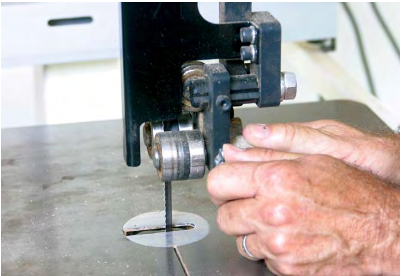
It is important that all the guides be adjusted properly. Better quality band saws feature roller-bearing guides.
