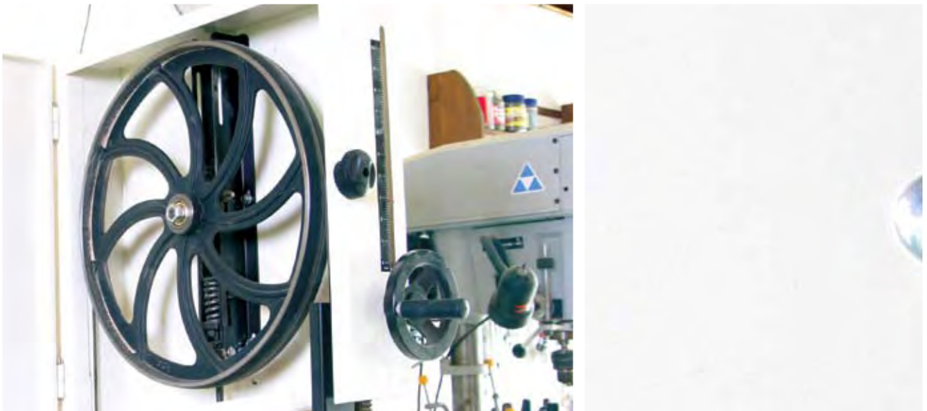
Band saw blades ride on rubber-covered wheels. It is important to have proper blade tension to match the blade width.
