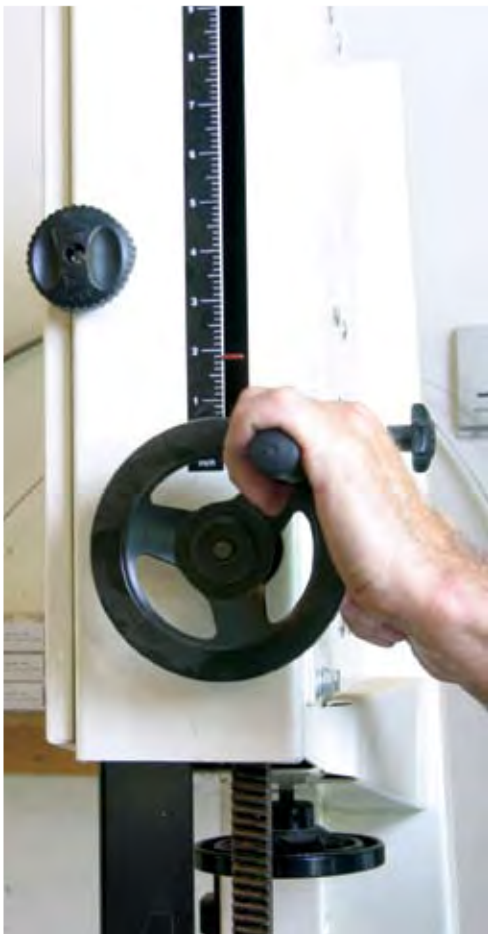
The blade guides are adjustable up and down to match the thickness of the stock being cut. Quality saws such as the Jet shown utilize a wheel for adjustment.
